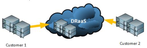
For a cloud service provider providing in the cloud hosting and disaster recovery (ICDR), where customer organization production is hosted by the cloud service provider and the cloud service provider offers disaster recover to another site.
