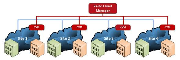
As can be seen in the diagram above, each site has a ZVM installed. One site has the Zerto Cloud Manager installed to manage all the sites.
